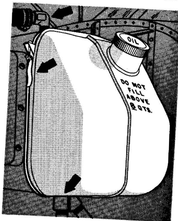
FIGURE 3-7. Oil tank inspection.
