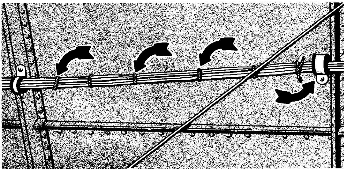
FIGURE 1-9. Proper routing of electrical wiring.
