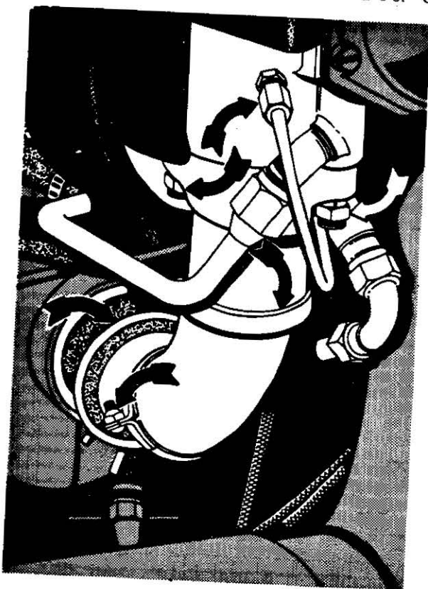
FIGURE 3-6. Intake manifold checkpoints.
